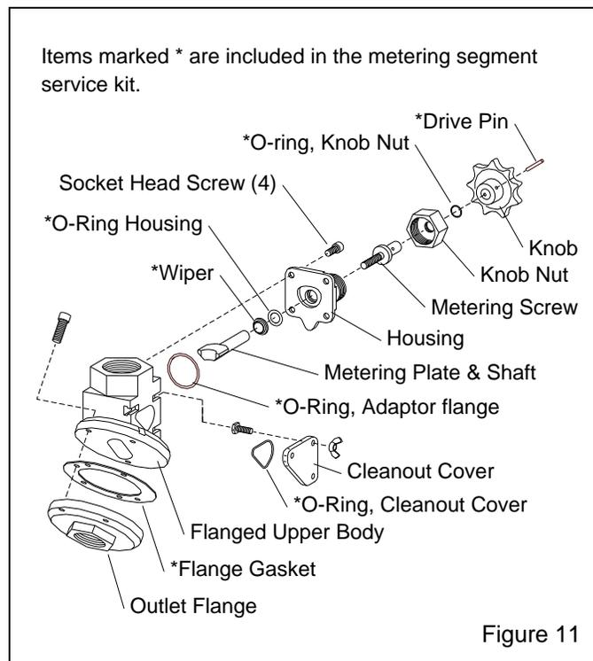
6.7.12 Thoroughly clean and inspect all parts that are to be reused. Replace all worn parts.
