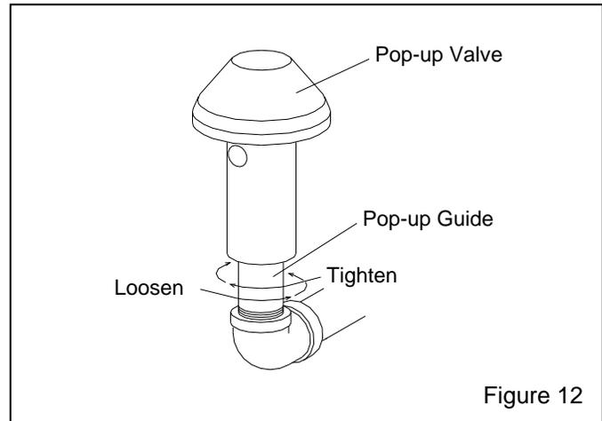
**6.8.6** Refer to Figure 13 to check the pop-up height. If the pop-up sits too low, misalignment could occur when the pop-up comes up against the seal. If the pop-up sits too high, it will take longer for abrasive to flow through the opening when filling. Adjust the height by replacing the guide with one that is longer or shorter.
