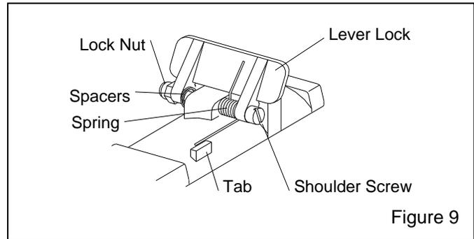
**6.6.2.2** Install a new lever lock and spring, and reassemble in reverse order.
