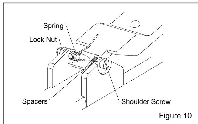
**6.6.3.2** Install a new handle lever and spring, and reassemble in reverse order.
